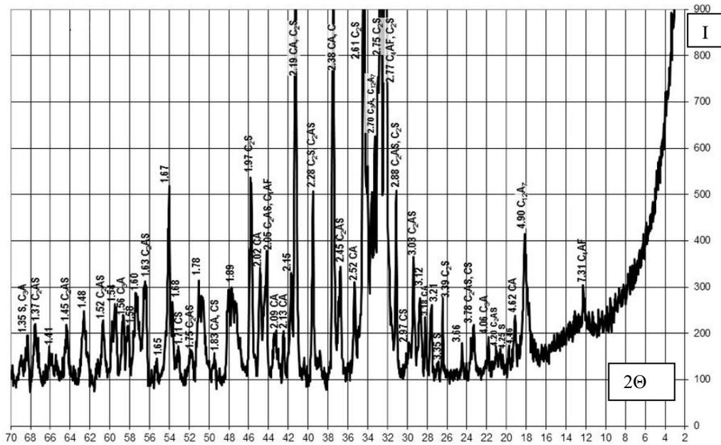
Figure 5. X-ray diffraction of clinker sample 2S (1200°C).
