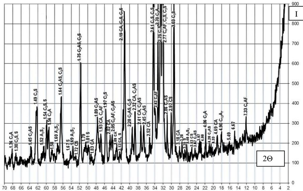
Figure 6. X-ray diffraction of clinker sample 2S (1400°C).
