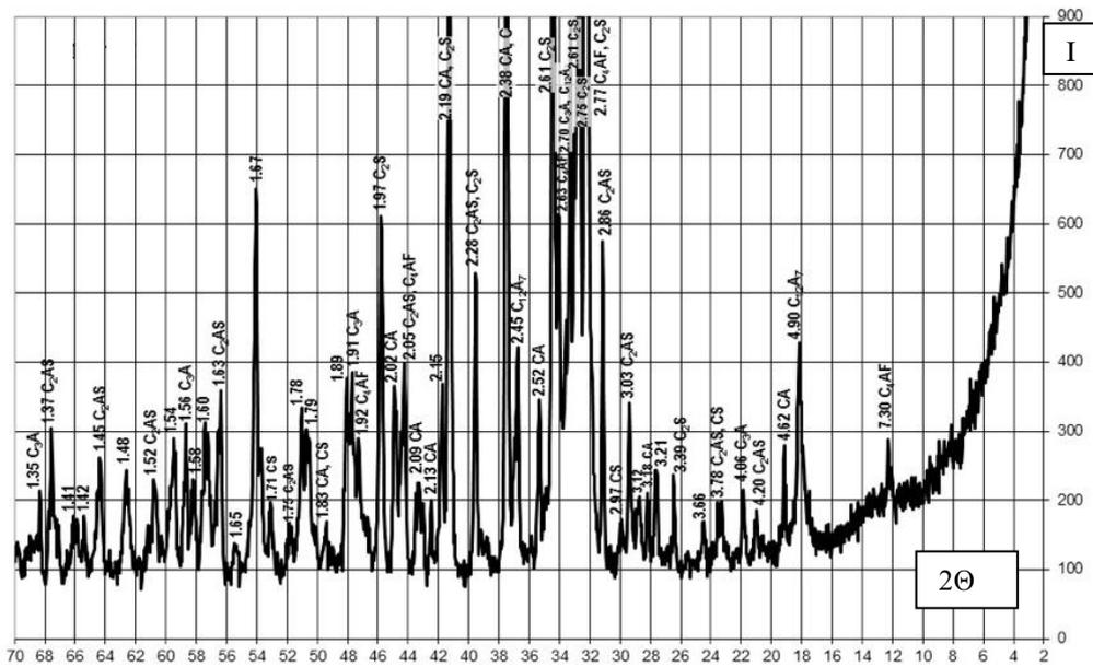
Figure 3. X-ray diffraction of clinker sample 1S (1200°C).
