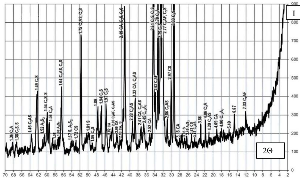
Figure 4. X-ray diffraction of clinker sample 1S (1400°C).
