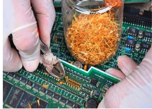
Figure 6. Precious metals in electronic boards (research laboratory, Italy, 2017).
