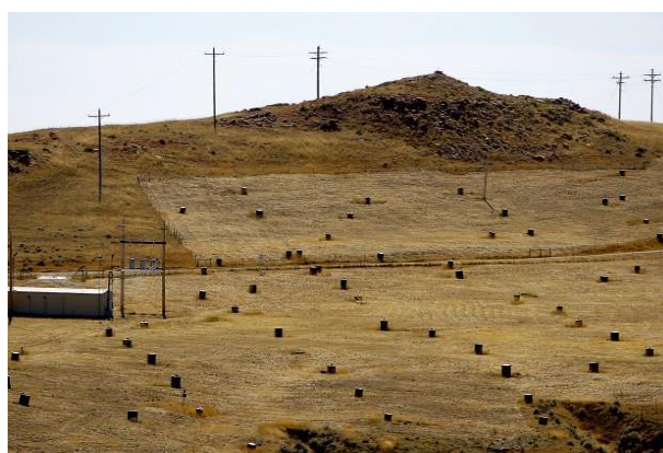
Figure 13. In-situ leaching method. Schematic representation of the process applied in the U.S.A. for the extraction of uranium (a) and example of practical application in Kazakhstan for the extraction of copper (b) [5-8].
