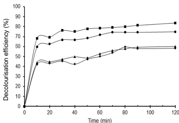
Figure 3. Effect of GOx dosage (0.05 g (▲); 0.07 g (■), 0.1 g (●), 0.3 g (◆)) on decolourisation of beet sugar syrup at 20 mM glucose, pH 7, and T= 30°C.
