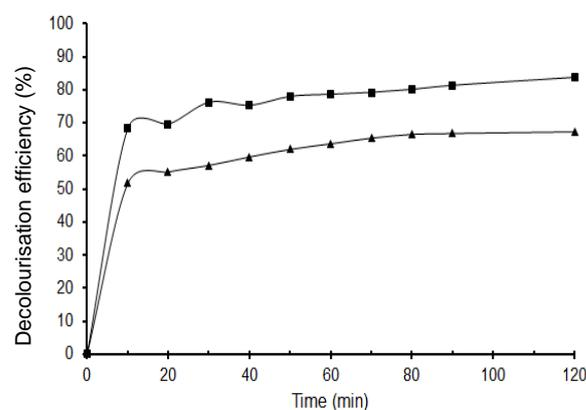
Figure 6. Decolourisation of beet sugar syrup with GOx-immobilized AC particles (■) and the combined AC/GOx (▲), 20 mM glucose, pH 7, and T= 30°C.
