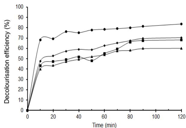
Figure 4. Effect of operating temperature (15°C (▲); 25°C (■), 30°C (●), 35°C (◆)) on decolourisation of beet sugar syrup, at 0.07 g GOx dosage, 20 mM glucose, and pH 7.
