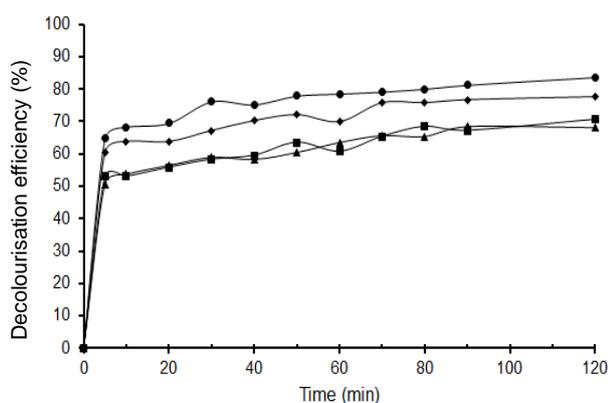
Figure 5. Decolourisation of beet sugar syrup by the combined AC/GOx process at various solution pH (pH 5 (▲); pH 6 (■), pH 7 (●), pH 8 (◆)), 0.07 g GOx dosage, 20 mM glucose, and T= 30°C.
