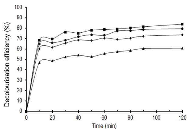
Figure 2. Decolourisation efficiency of beet sugar syrup at various concentrations of glucose (15 mM (▲); 20 mM (■), 25 mM (●), 30 mM (◆)) 0.07 g GOx dosage, pH 7, and T= 30°C.
