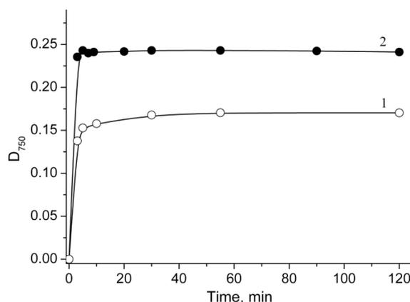
**Figure 5.** Change in D<sub>750</sub> value during Folin-Ciocalteu test for the CA+A300 composite (curve 1) and for an equivalent quantity of individual CA (curve 2).
