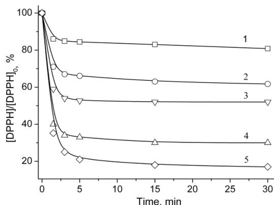
**Figure 2.** Inhibition of DPPH<sup>•</sup> radicals in the reaction with CA solutions at a molar  $[CA]/[DPPH^{\bullet}]$  ratio of 0.05; 0.075; 0.10; 0.15; 0.30 (curves 1-5, respectively).
