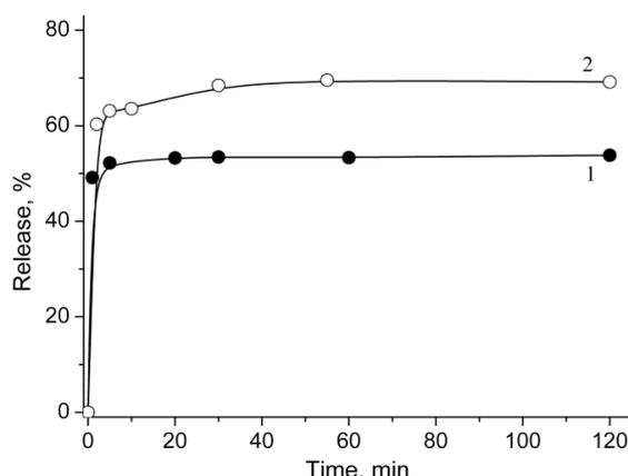
**Figure 7. Percentage of CA released from the composite into pure water (curve 1) and into the reaction mixture of the Folin-Ciocalteu test (curve 2).**
