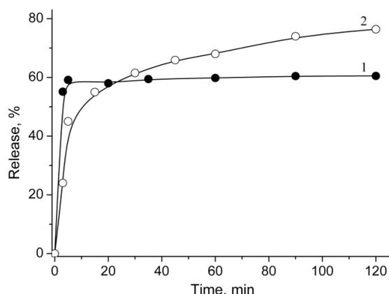
**Figure 6. Percentage of CA released from the composite into 70 % ethanol (curve 1) and into the reaction mixture of the DPPH<sup>•</sup> test (curve 2).**
