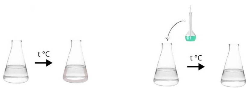
Figure 1. Scheme of the water treatment process with antiscalant RT-2024-4 for scale removal.
